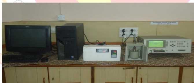
Fig.3 LCR meter and sample holder for the measurement of AC conductivity
